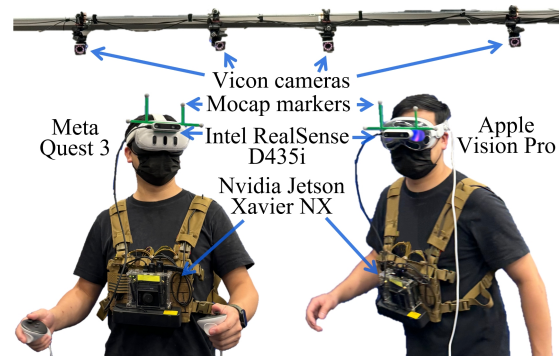
Figure 1: Our XR headset tracking performance testbed.
