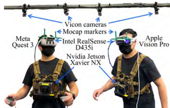
Figure 1: Our XR headset tracking performance testbed.
